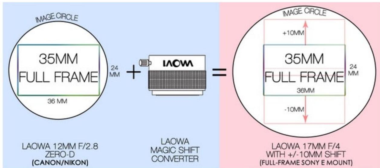
THE OPTICS IN THE MAGIC CONVERTER EXPAND THE IMAGE CIRCLE BY 10MM
